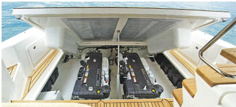
Engine access for the Volvo Penta IPS pod drives is as easy as pushing a button to raise the cockpit floor.
