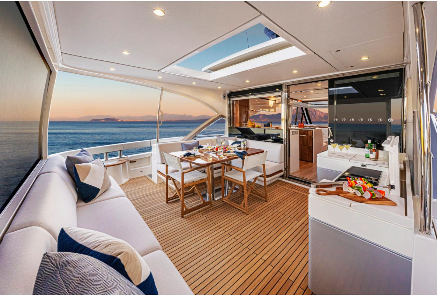
**Above:** The cockpit has room for 10 people on two settees, along with a barbecue grill, refrigerator drawers and a folding dining table. A hardtop protects the area from the sun, with tinted glass quarter panels and an electrically retractable blind that shields the after section. **Below:** The full-beam, amidships master stateroom.
